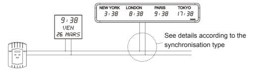
The clock can be synchronised via a radio antenna or an IRIG B/AFNOR network.
