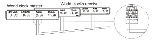
An independent clock can synchronise another IRIG B / AFNOR receiver. Connect the 2 wires for the IRIG B/AFNOR signal to terminal block (L) on the transmitting World clock, as well as to terminal (L) on the world receiver clock.
